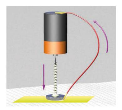
Challenge: Make a spinning propeller out of a homopolar motor with house-hold objects by manipulating its magnetic fields.
